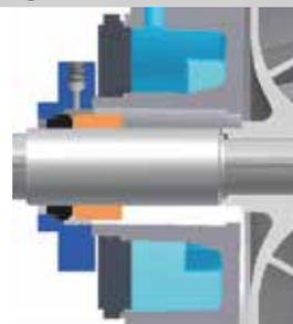
**A (E) single seal with flushing + bottom ring**
