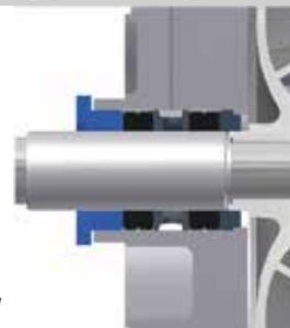
**L double tandem mechanical seal**
