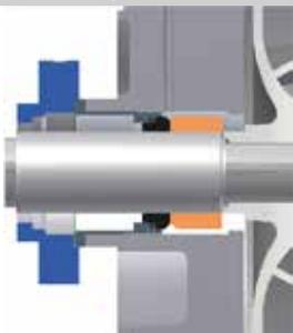
**B (S) gland packing (with flushing)**
