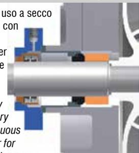
**U single seal close to the impeller**
